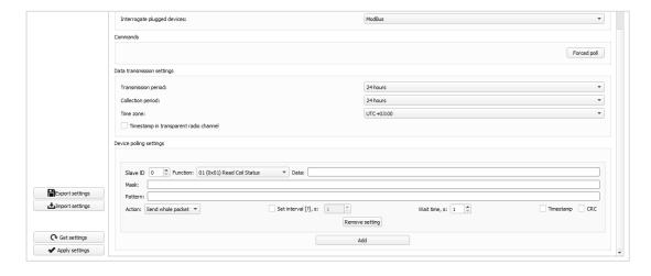
Slave ID – address of the connected device.
