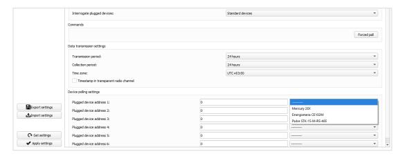
ModBus RTU. Data exchange with the device connected to the Vega SI-13 takes place using the ModBus RTU protocol. If necessary, this mode can be configured using the "Add" button. In the drop-down menu, you can configure the following settings:
