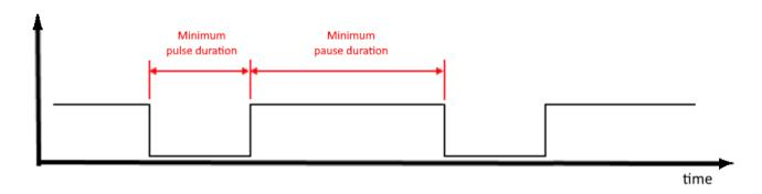
3. In addition to filtering pulses by the duration of the pause and pulse, the modem provides the ability to filter the pulse by rising and falling. For detailed settings, refer to the group of parameters for clamping pulses at the inputs. The available values are "make" (falling), "open" (edge), or "make and break".
