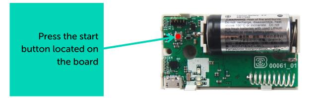
**2. OTAA.** After pressing the start button, the device makes three attempts to connect to the network within the set frequency plan. After the activation request confirmed by LoRaWAN network, the device sends a signal and switches to the "Active" mode. If all attempts fail, the sensor will continue to accumulate data and will attempt to connect to the network every 6 hours.
