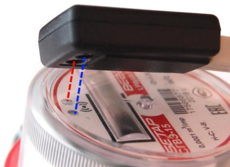
Figure 8 — "Opticalport-USB" adapter location in relation to meter_Close-up
