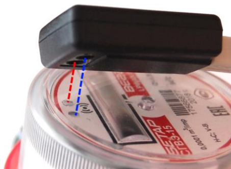
Figure 8 — "Opticalport-USB" adapter location in relation to meter_ Close-up
