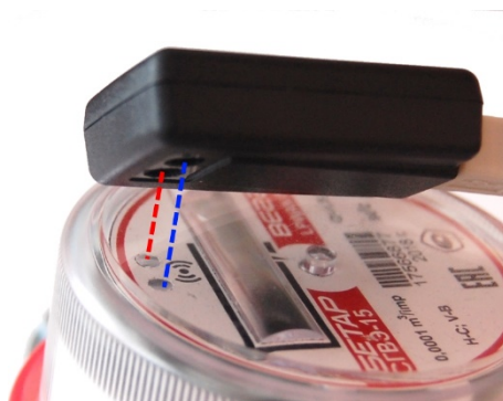
Figure 8 — “Optical port-USB” adapter location in relation to meter_ Close-up
